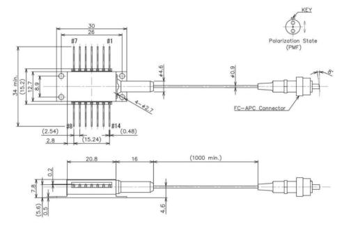
(a) 900um fiber diameter and FC/APC connector type (QLD106L-6430)
